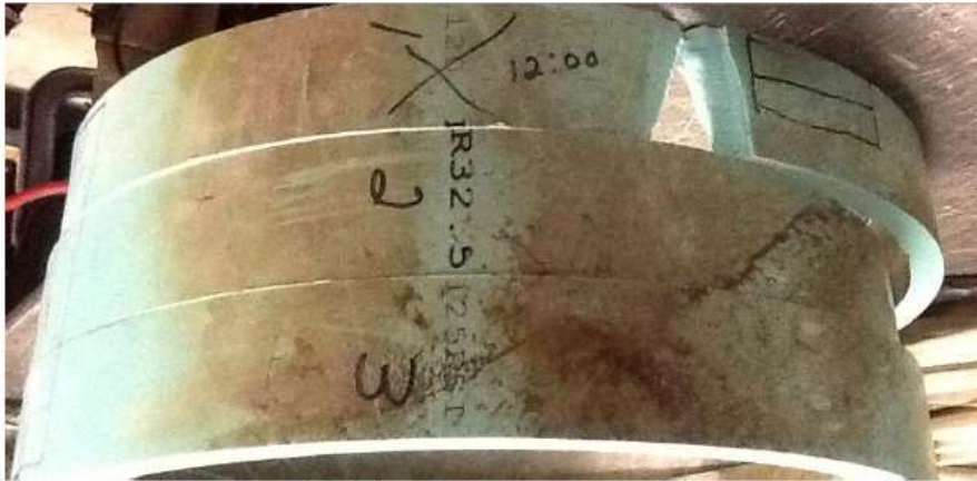
Figure 6. Photograph of the three test rings following completion of the ASTM D2412 compression test. One of the three rings (top) fractured with expulsion of a triangular shaped piece.
